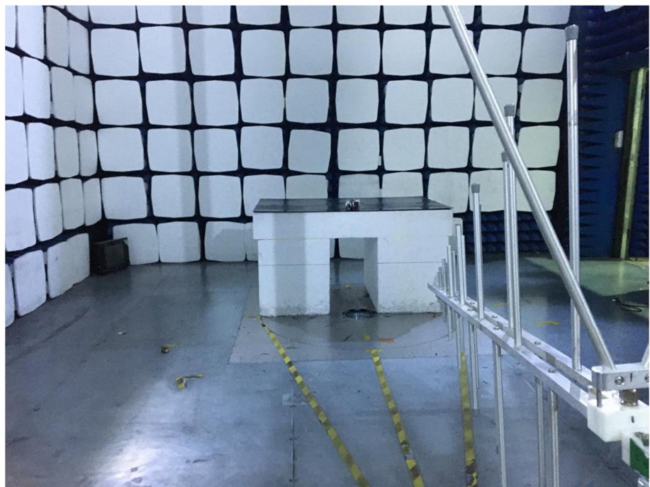
Radiation Emission Test Setup (30MHz to 1GHz)
