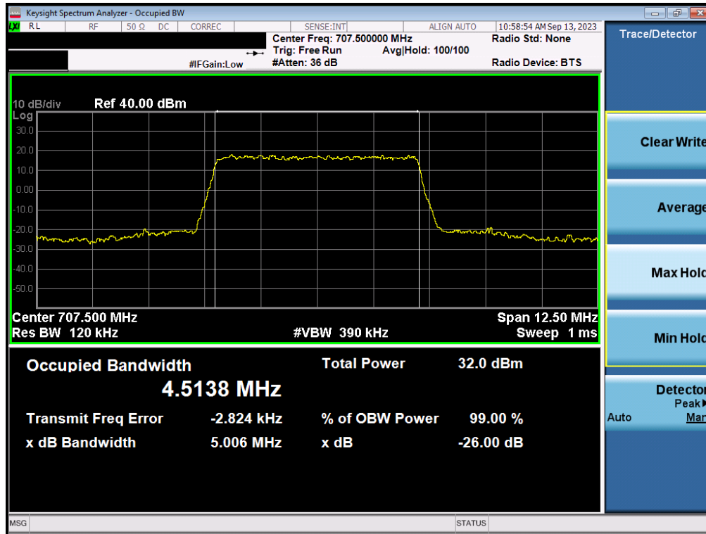
Plot 7-11. Occupied Bandwidth Plot (LTE Band 12 - 5MHz QPSK - Full RB – ANT1)
