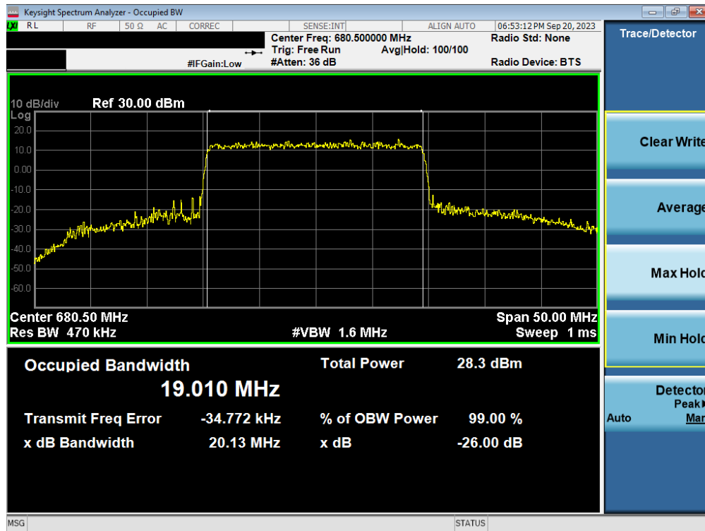
Plot 7-23. Occupied Bandwidth Plot (NR Band n71 - 20MHz CP-OFDM 16-QAM - Full RB – ANT1)
