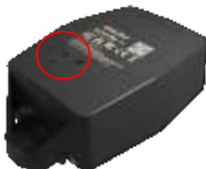
Figure 1 – Hati Location of the indicator for magnet switch (detector)
