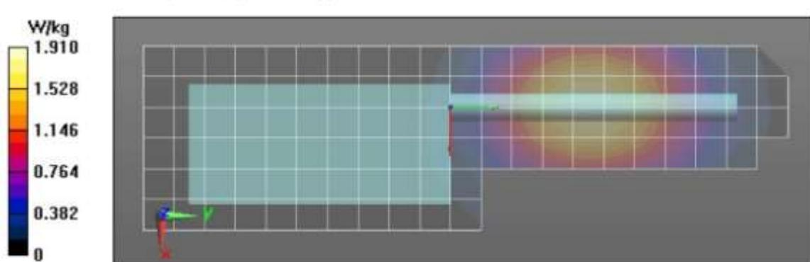
**Shortened scan reflects highest SAR producing configuration and is compared to the full scan.**
