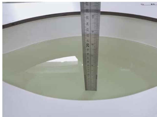
Liquid depth in the body phantom (2450MHz)
