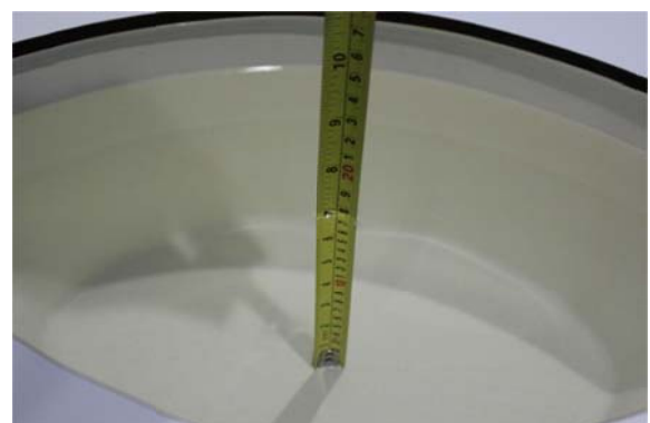
Liquid depth in the body phantom (2600MHz)
