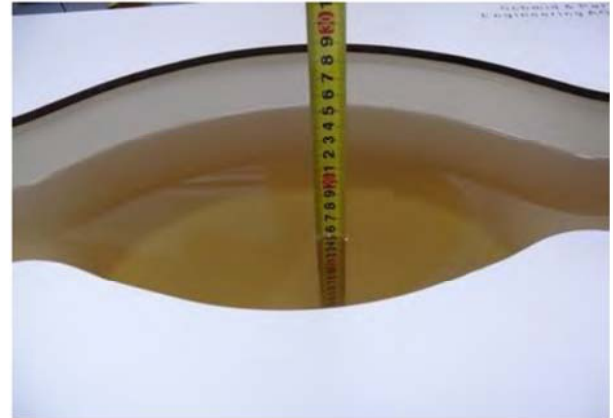
Liquid depth in the body phantom (835MHz)
