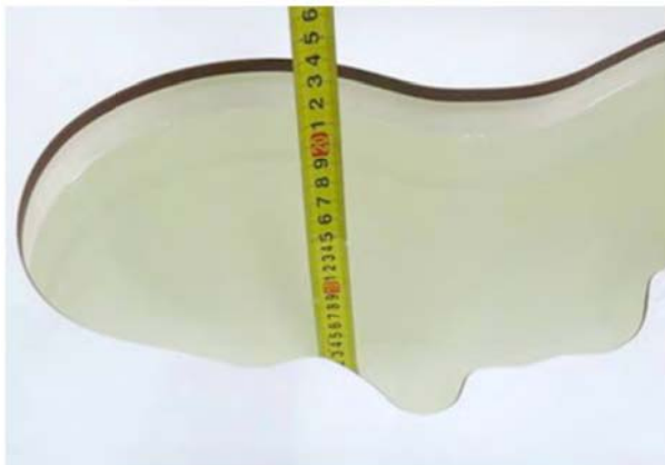
Liquid depth in the head phantom (835MHz)
