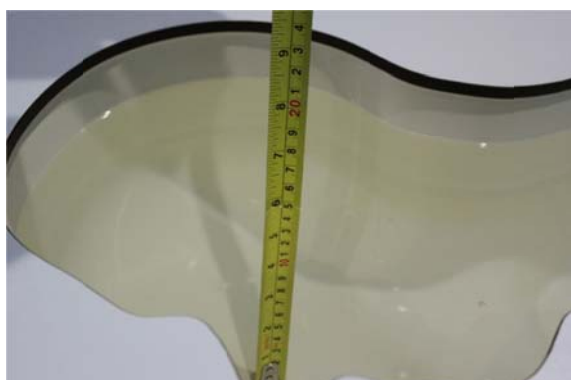
Liquid depth in the head phantom (2600MHz)
