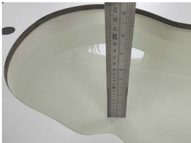
Liquid depth in the head phantom (2450MHz)
