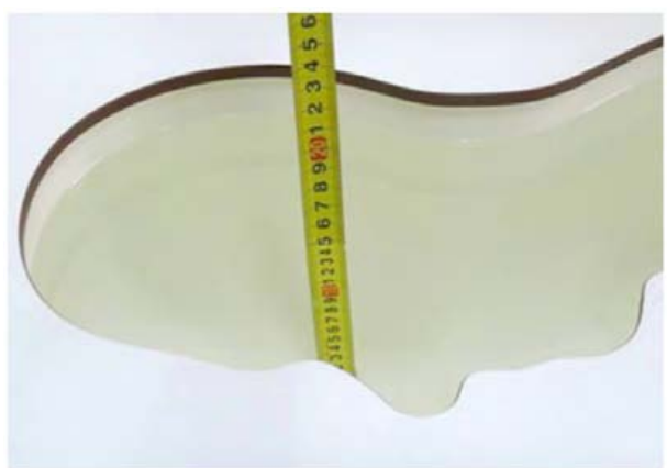
Liquid depth in the head phantom (835MHz)
