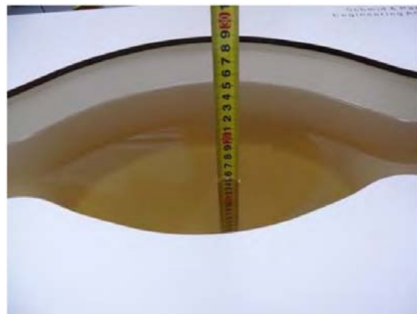
Liquid depth in the body phantom (835MHz)
