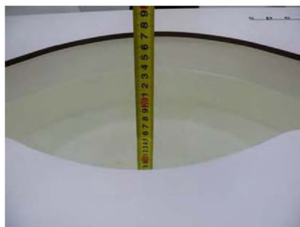
Liquid depth in the body phantom (1900MHz)
