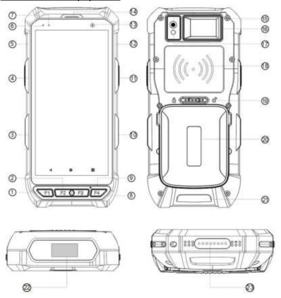
①F1 ②F2 ③Volume ④Reserved Button ⑤USB port ⑥Blue Led Indicator ⑦Red LED indicator ⑧F3 ⑨F4 ⑩Power Button ①Reserved Button ②Reserved Pogo Pin ③Front Camera ④Receiver ⑤Rear Camera ⑥Label ⑦Flashlight ⑱RFID Reading Area ⑨Battery Cover Locker ②Battery Cover ②Wrist Strap Locker ②Barcode Scan Window ③Cradle Pogo Pin Connector
