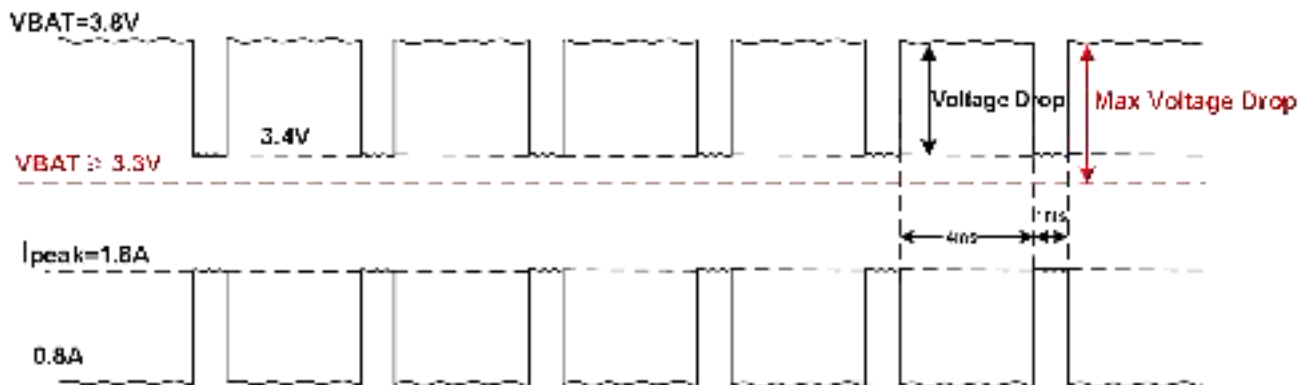
Figure 4: Power consumption at ENDC combination of B2 (20MHz) and N79 (100MHz)
