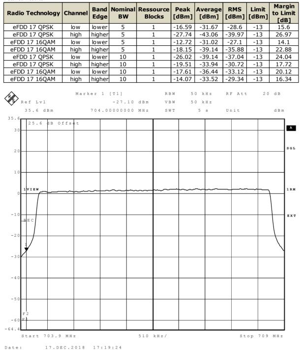
eFDD17 16QAM 5MHz Channel = LOW
