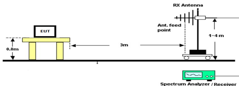
Radiated Test Setup, Above 1000 MHz
