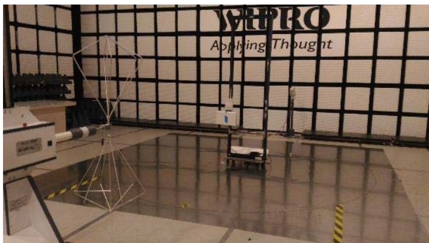
Figure 6 Test setup for Radiated Emission test from 30MHz to 200MHz - Vertical Polarization
