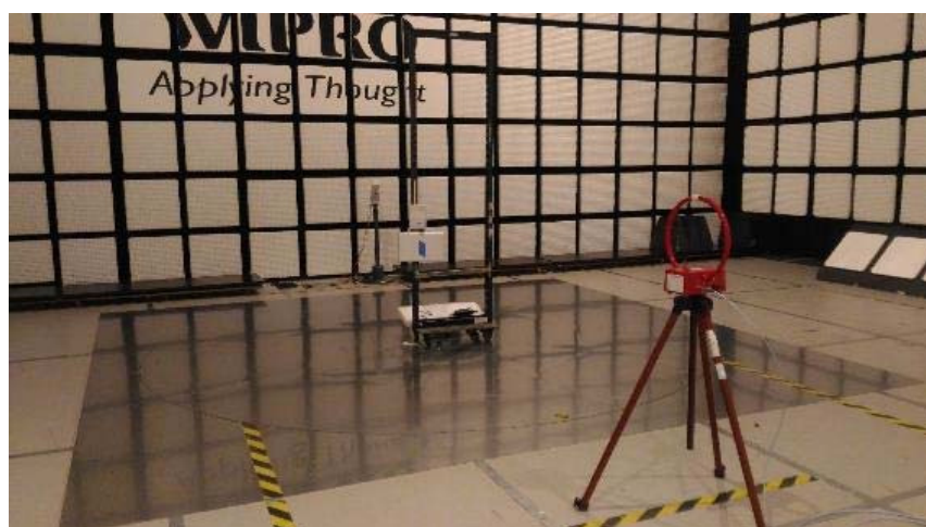
Figure 4 Test setup for Radiated Emission E field measurement from 9 kHz to 30MHz – Perpendicular
