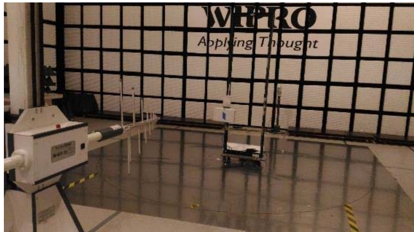
Figure 8 Test setup for Radiated Emission test from 200MHz to 1GHz -Vertical Polarization
