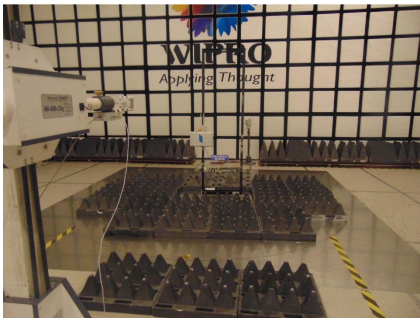
Figure 13 Test setup for Radiated Emission test from 26.5GHz to 40 GHz – Horizontal Polarization
