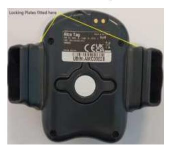
The Locking Pates will be secured in position when the Strap is inserted into the Alco Tag, they protect the strap from being released without physical damage being created for evidence gathering purposes.
