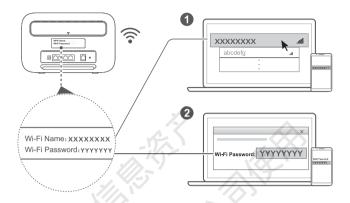
Once the router has connected to a mobile data network, you can connect your computer or mobile phone to the router's Wi-Fi network to access the Internet. Please refer to the label on the back of the router for the default Wi-Fi network name (Wi-Fi Name) and password (Wi-Fi Password).
