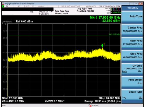
Spurious / Simultaneous / Downlink / 27 GHz ~ 40 GHz
