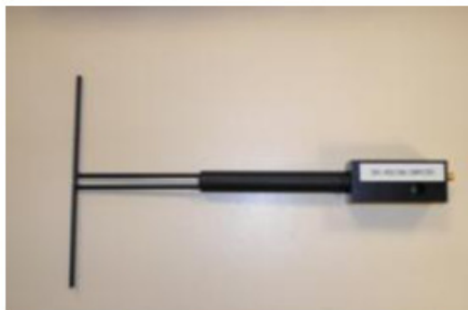
Figure 1 – Satimo COMOSAR Validation Dipole
