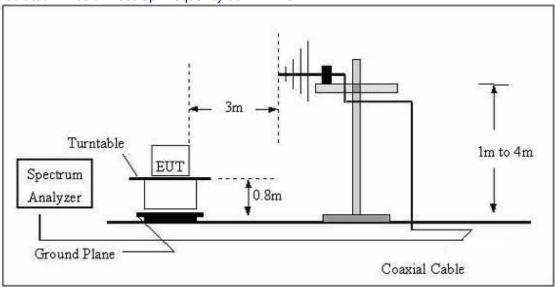
(C) Radiated Emission Test-Up Frequency Above 1GHz
