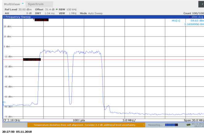
Figure 8.5-1: 2172.5 and 2177.5 MHz AGC -0.5 Upper Edge Out-of-block
