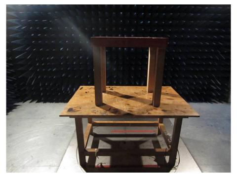
1.5M-HEIGHT TEST TABLE FOR RADIATED EMISSION TEST SETUP (ABOVE 1 GHz)
