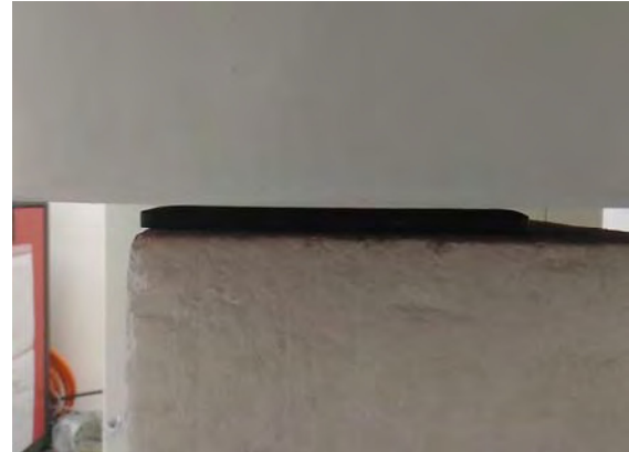
Fig.3 EUT Back side to flat phantom
