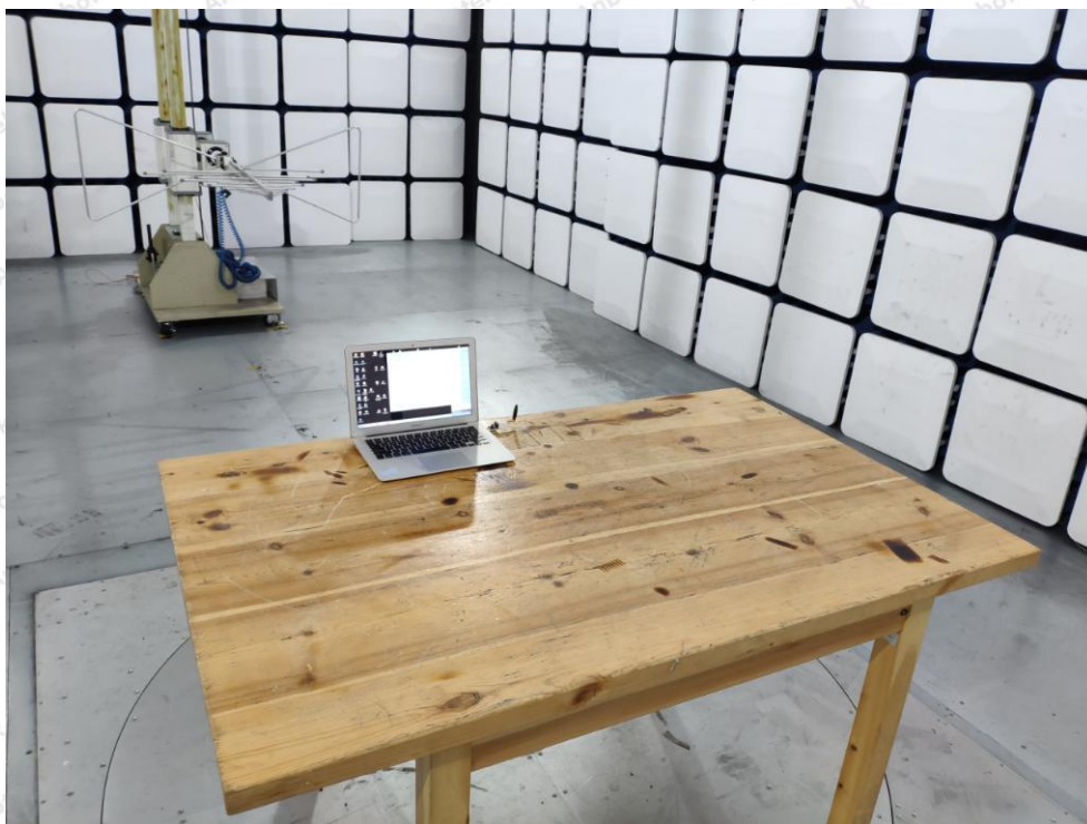
Photo of Radiation Emission Test
