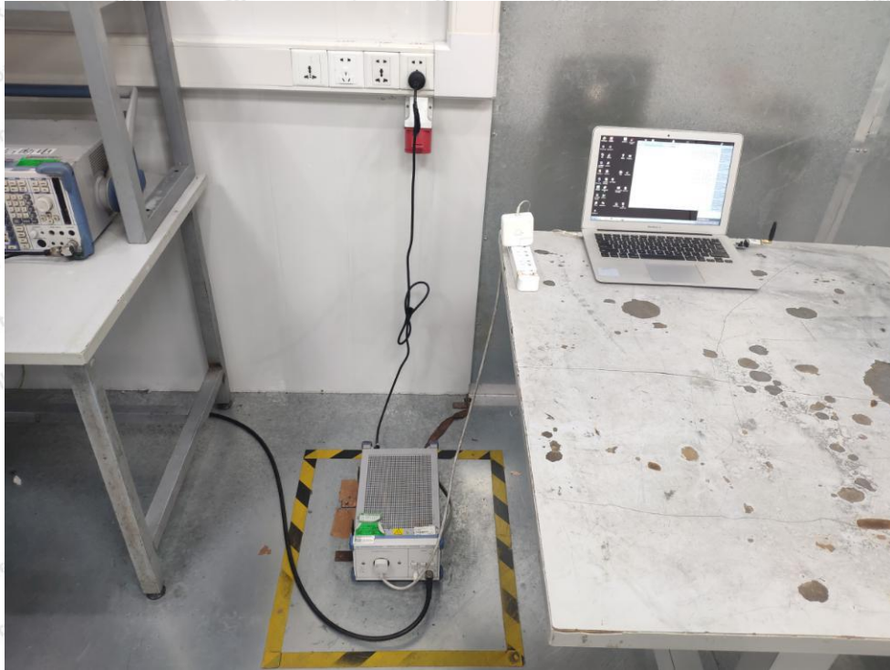
Photo of Radiation Emission Test
