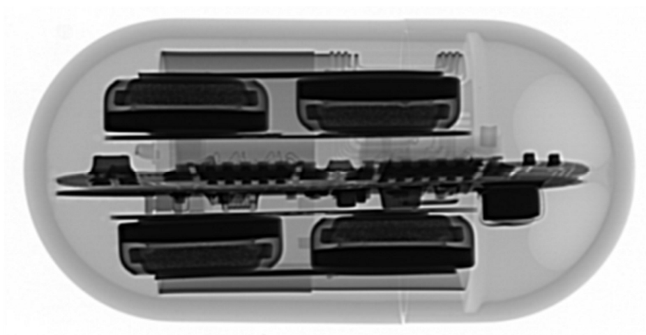
Folded PCB – fitted to capsule
