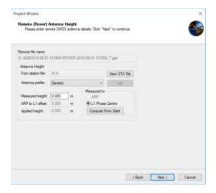
For base data, IE supports two options to load: First is from base station and second is download via PPP mode. Also, the precise file can also be downloaded to improve accuracy. Click Next.
