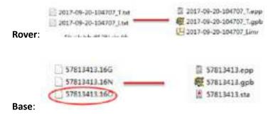
**Notice**: When convert rover files, double click IMU file and select **SPAN Model** as **SPAN KVH1750**.
