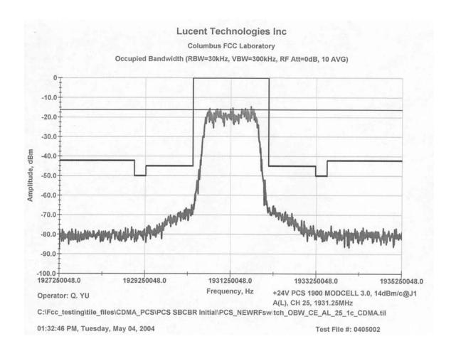
PCS A-Band, Lower Edge Channel Channel 25, 1931.25 MHz Measured at the output of SBCBR transceiver
