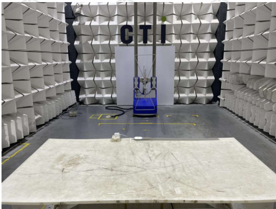
Radiated spurious emission Test Setup-1(Below 1GHz)
