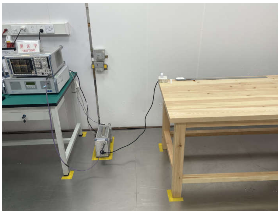
Conducted Emissions Test Setup
