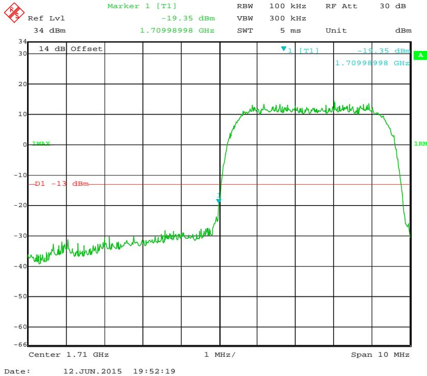
**AWS Band, Right Band Edge for HSDPA (16QAM) Mode**
