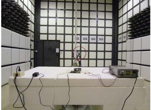
Radiated Emission Set up Photos (Below 1GHz)\_PCB Antenna
