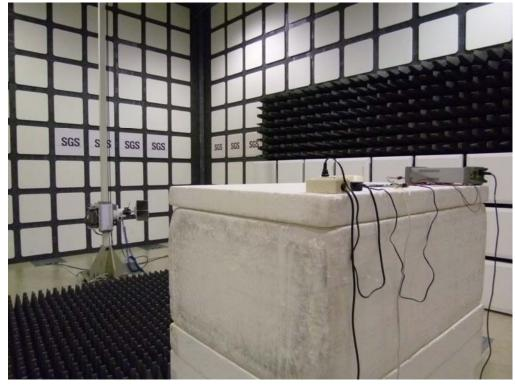
Radiated Emission Set up Photos (Front View)\_ROD Antenna
