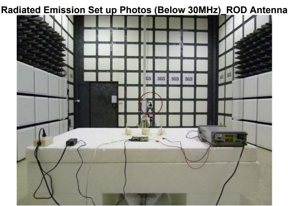
Radiated Emission Set up Photos (Below 1GHz)\_ROD Antenna
