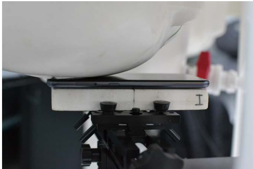
SAR Test Setup Photo 1 Right Cheek
