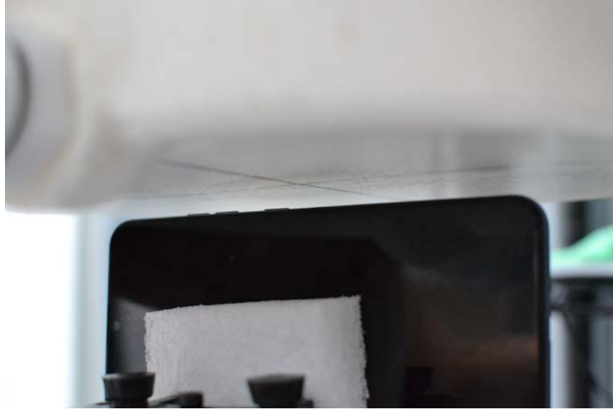
SAR Test Setup Photo 14 Right Edge 10 mm
