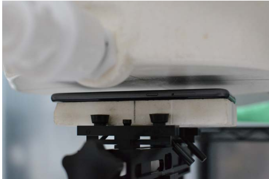
SAR Test Setup Photo 5 Back Side 10 mm
