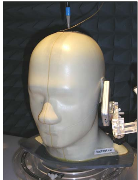
Figure 28: Positional Photograph of the Sagem A2005sca+ Handset in LH 15° Position (SAR Head Test)
