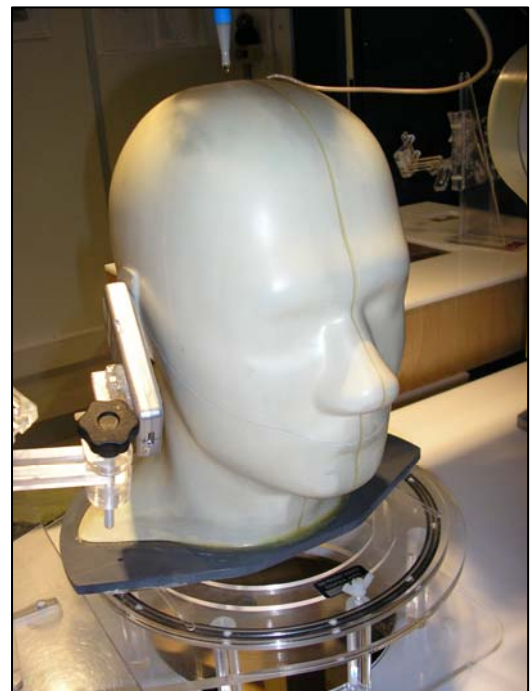
Figure 30: Positional Photograph of the Sagem A2005sca+ Handset in RH 15° Position (SAR Head Test)
