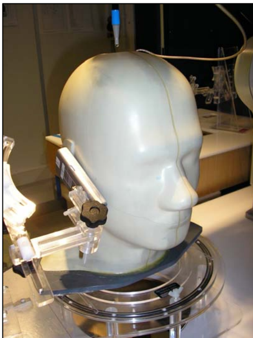
Figure 29: Positional Photograph of the Sagem A2005sca+ Handset in RH Cheek Position (SAR Head Test)
