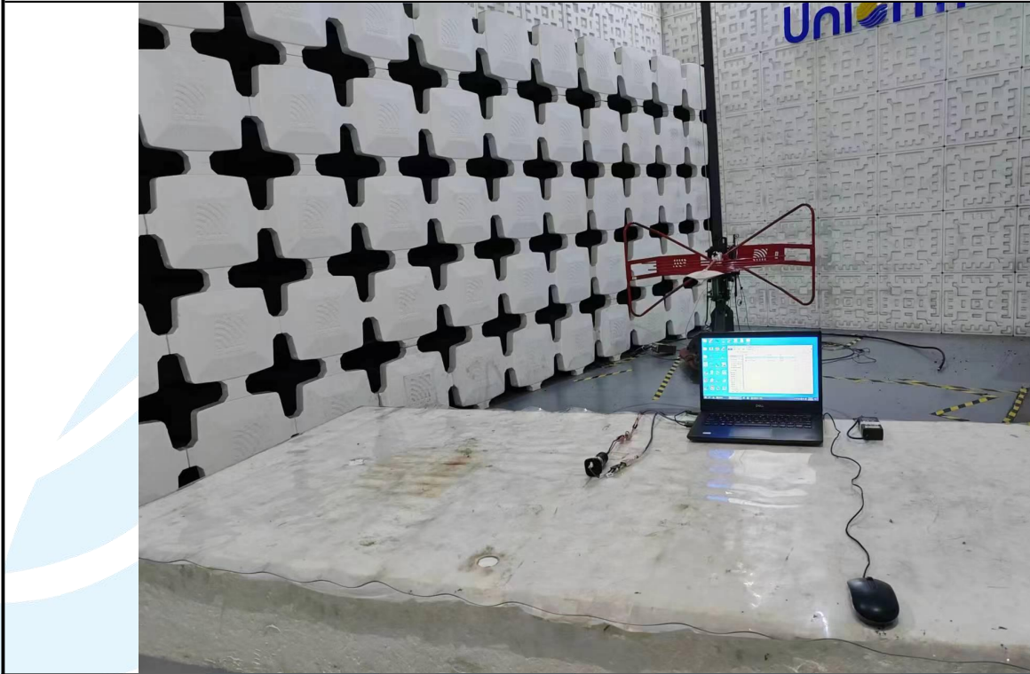
Radiated emission Test Setup (30 MHz~1 GHz)
