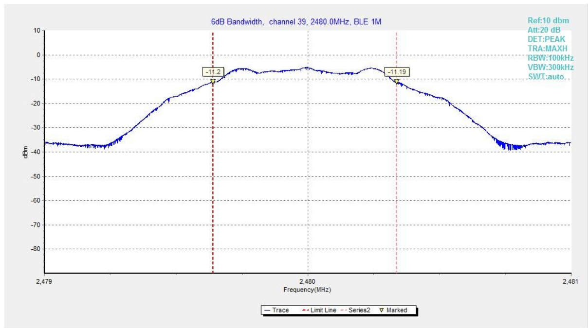
Fig.9 6dB Bandwidth (Ch 39), LE 1M
