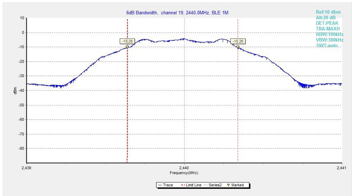
Fig.8 6dB Bandwidth (Ch 19), LE 1M
