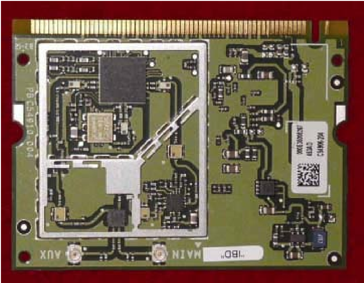
Front with Shielding Removed
