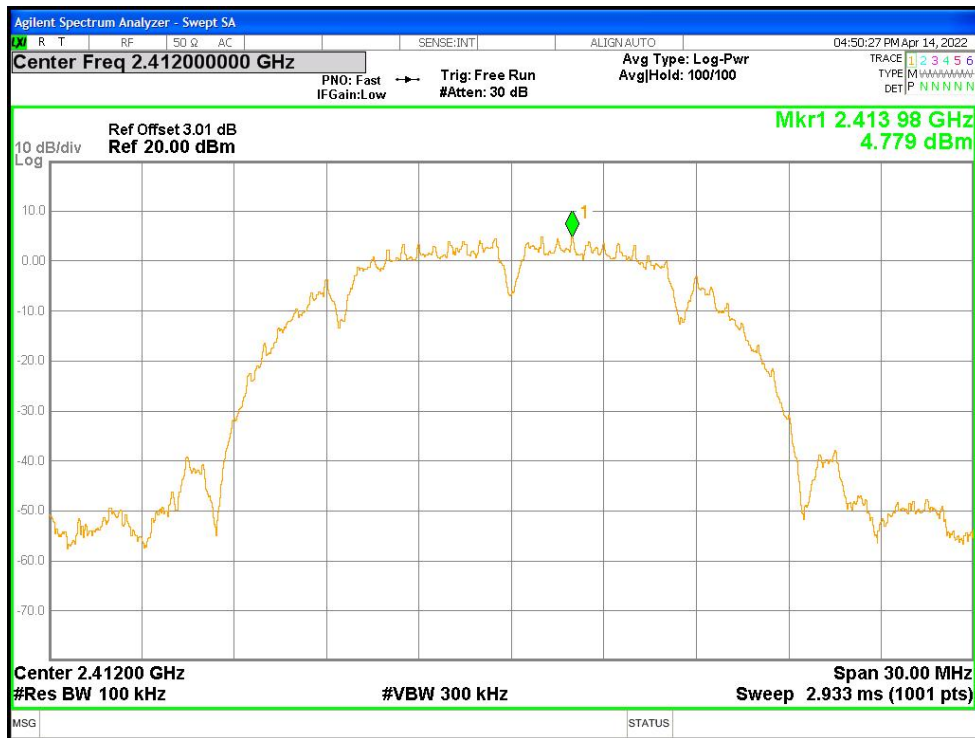
Tx. Spurious NVNT b 2412MHz Ant1 Emission
