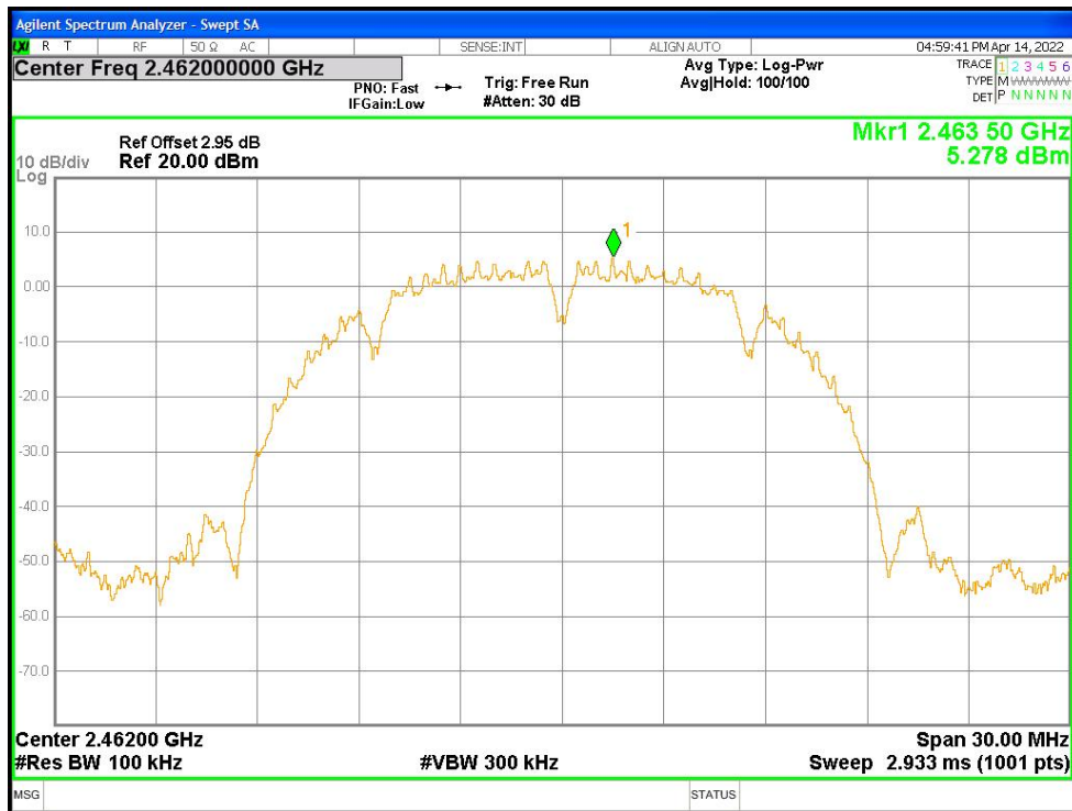
Tx. Spurious NVNT b 2462MHz Ant2 Emission
