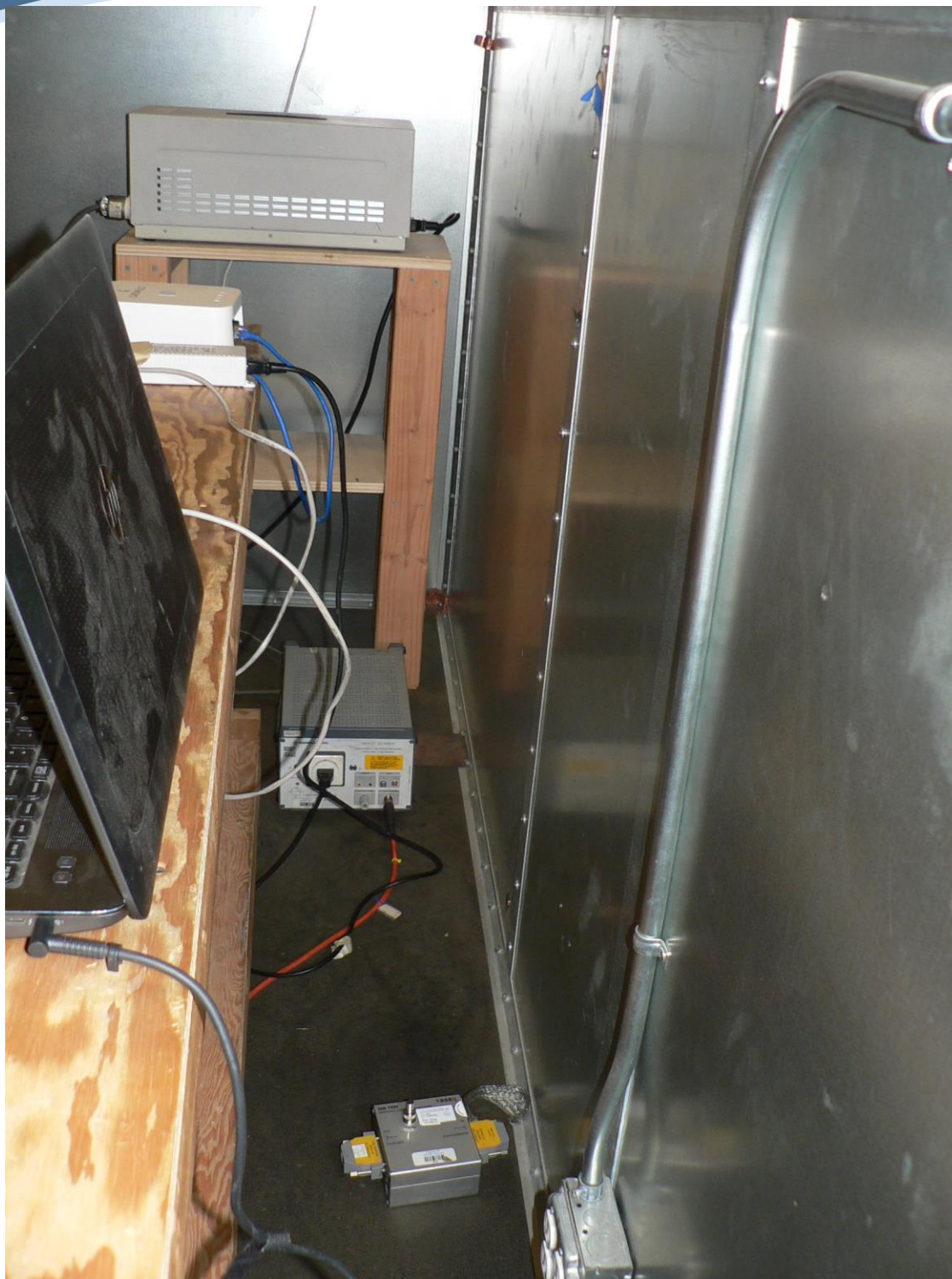
CATA04 AC Mains Conducted Emissions Side
