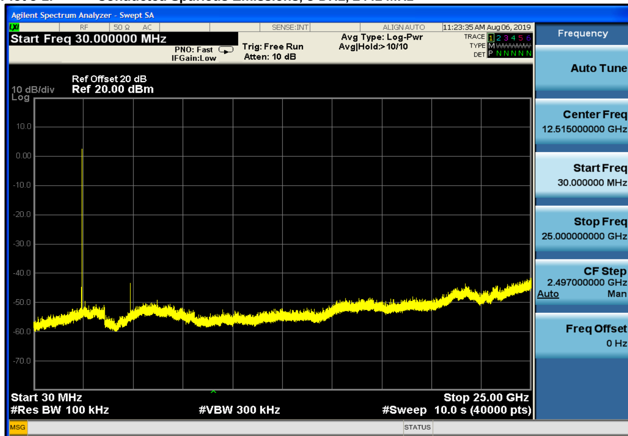
Plot 5-1: Conducted Spurious Emissions, 3-DH1, 2441 MHz
