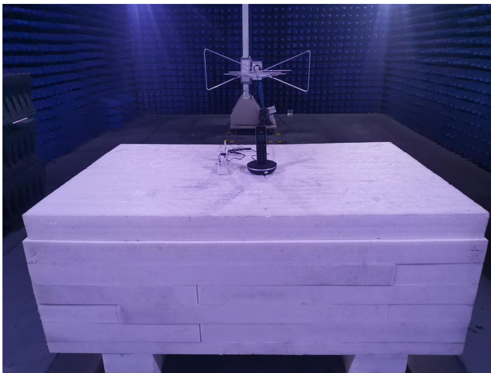
Photo of Radiated Emission Measurement (Above 1G)
