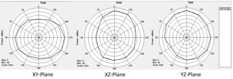
\* Antenna gain data were measured by UI chamber
