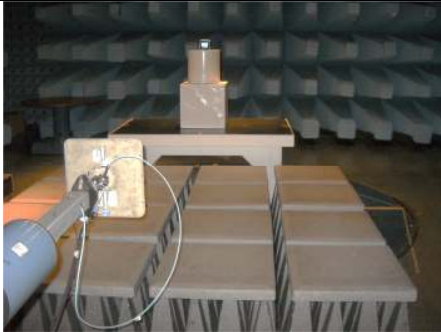
Radiated emissions set-up for frequencies above 1 GHz
