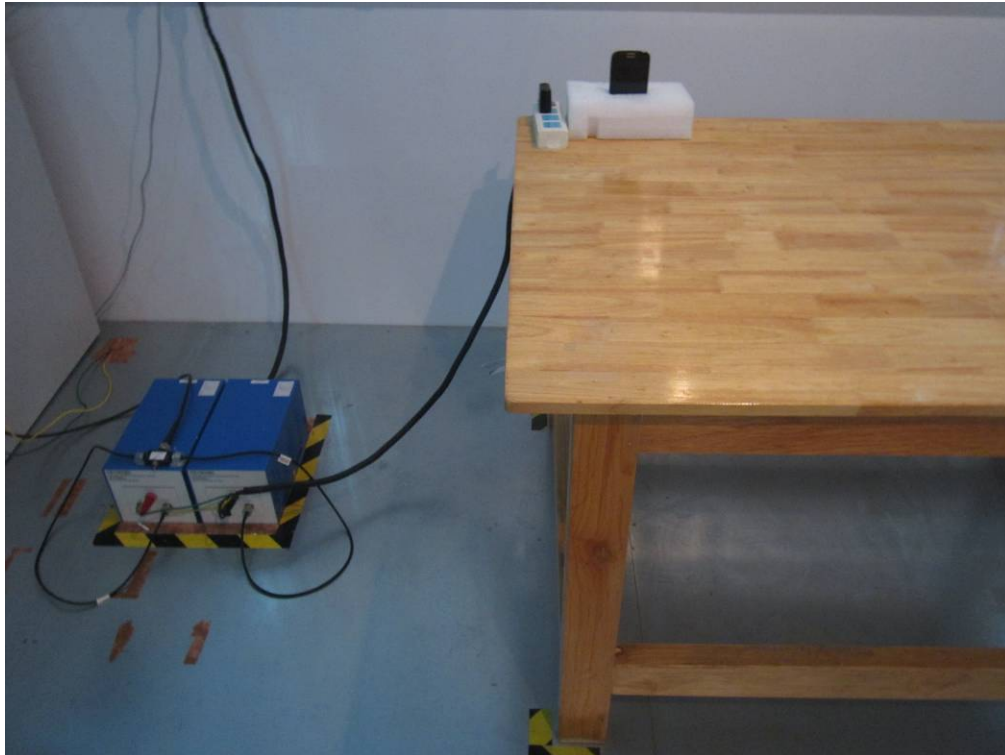
Conducted Emissions Test Setup Front View
