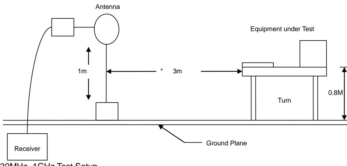
30MHz- 1GHz Test Setup
