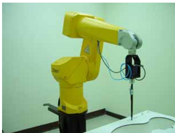
Fig. 5.2 Probe setup on robot
