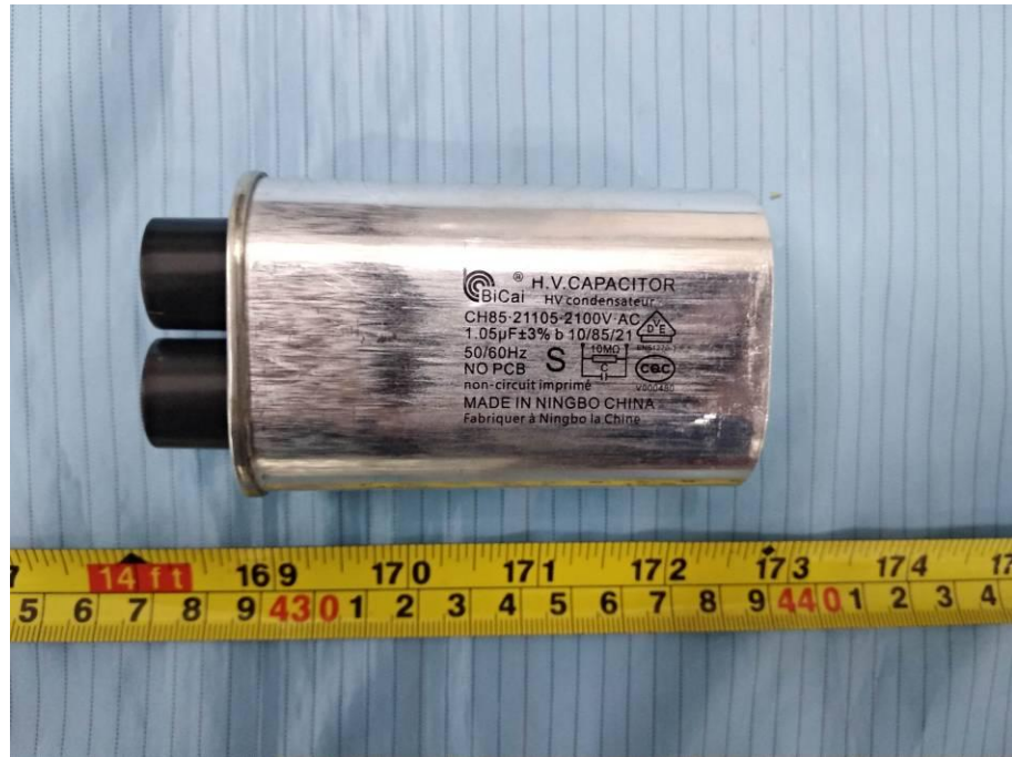
EUT – H.V. Capacitor Front View
