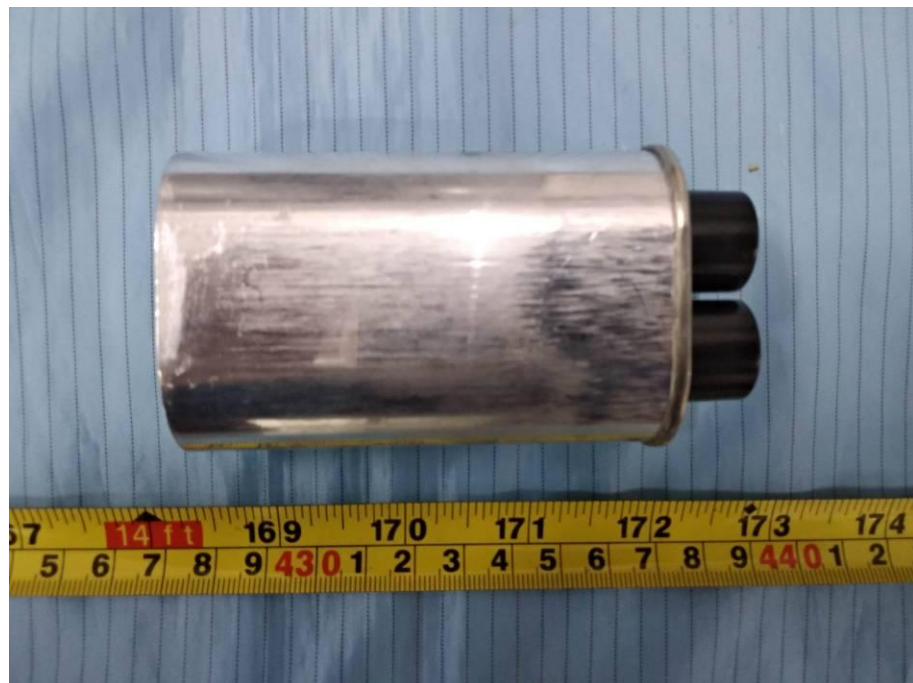
EUT – H.V. Capacitor Rear View
