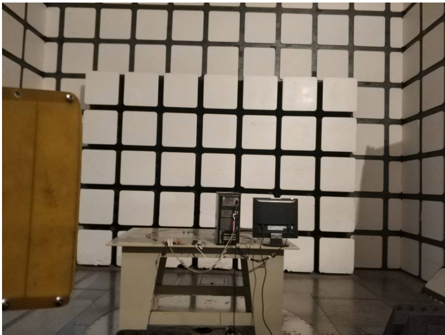
Radiated Emissions – Rear View (Above 1 GHz)
