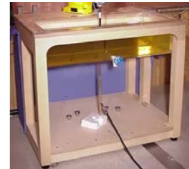
Validation Planar Phantom
