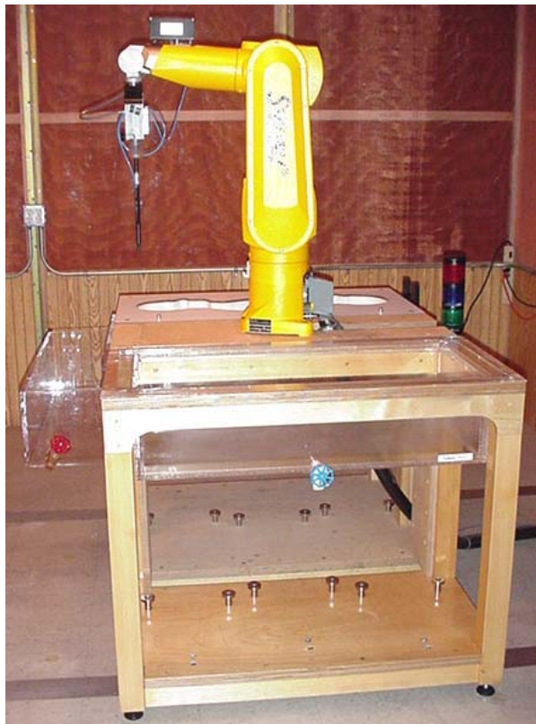
DASY4 SAR Measurement System with validation phantom
