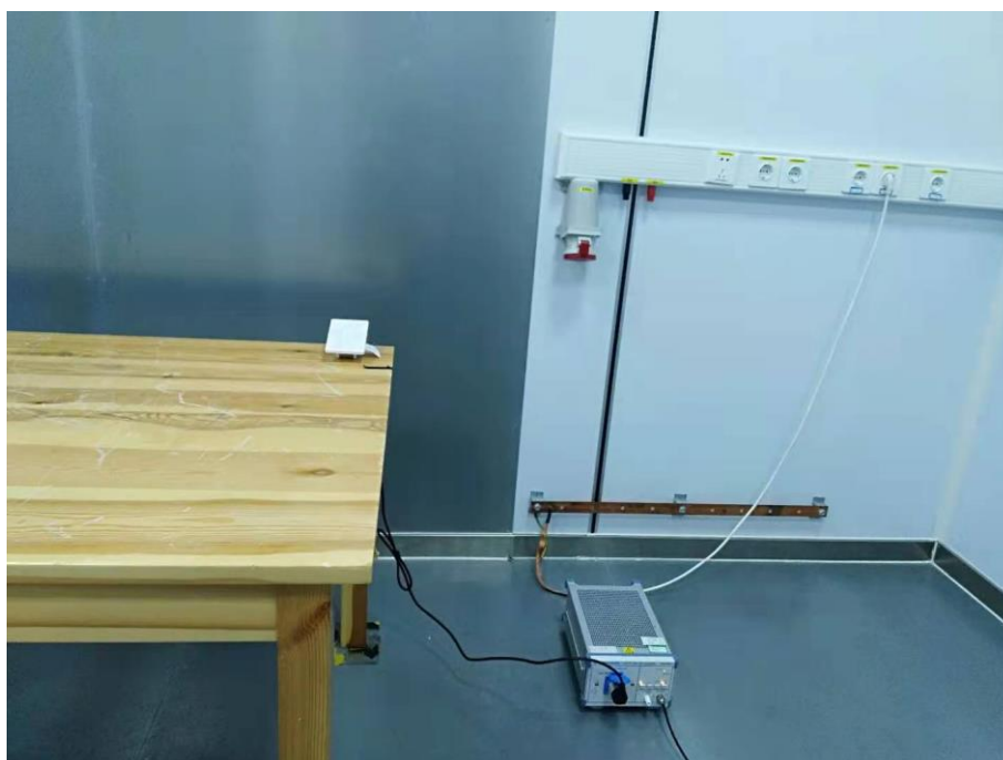
Fig. 4 Power line conducted emission setup photo
