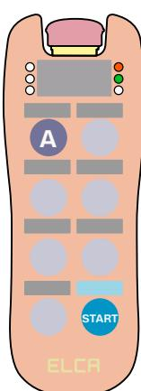
The white LEDs 1, 2 and 3 come on progressively depending on the charge status of the battery; if only LED 3 is on it indicates that the battery is low, LED 1, 2 and 3 on indicate that the battery is fully charged.
