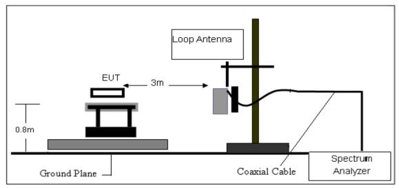
2. Radiated Emission Test-Up Frequency 30MHz~1GHz
