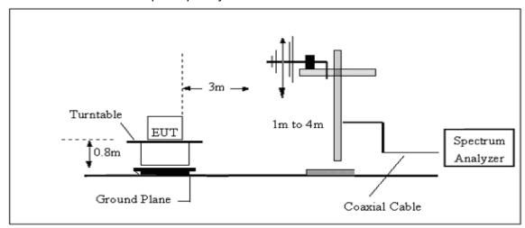
3. Radiated Emission Test-Up Frequency Above 1GHz
