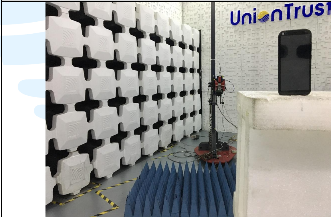
Radiated emission Test Setup (Above 1 GHz)
