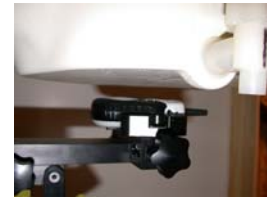
Figure 14.2 Face SAR Test Setup -- FRS --
