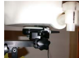
Figure 14.2 Body SAR Test Setup -- FRS --
