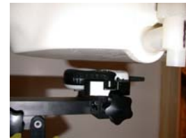
Figure 14.1 Face SAR Test Setup -- GMRS --
