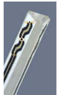
Figure 3.2 Probe Thick-Film Technique
