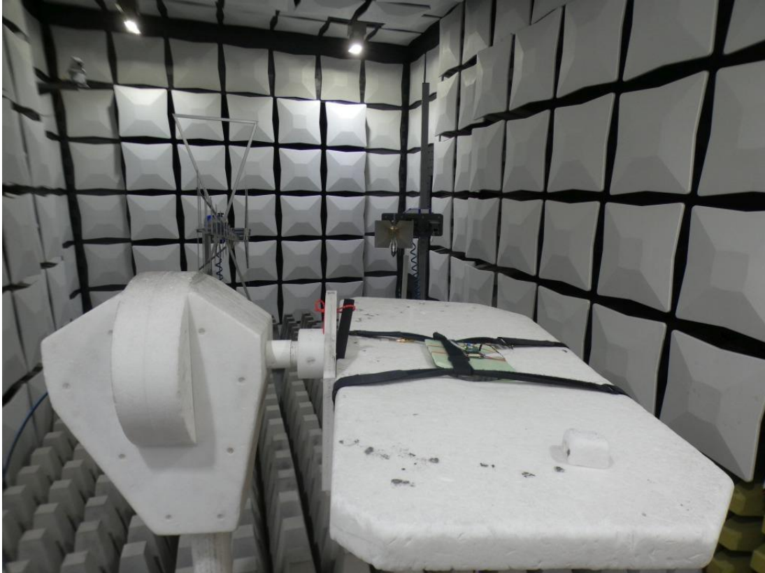
Photo 3: Test setup for radiated measurements above 26 GHz
