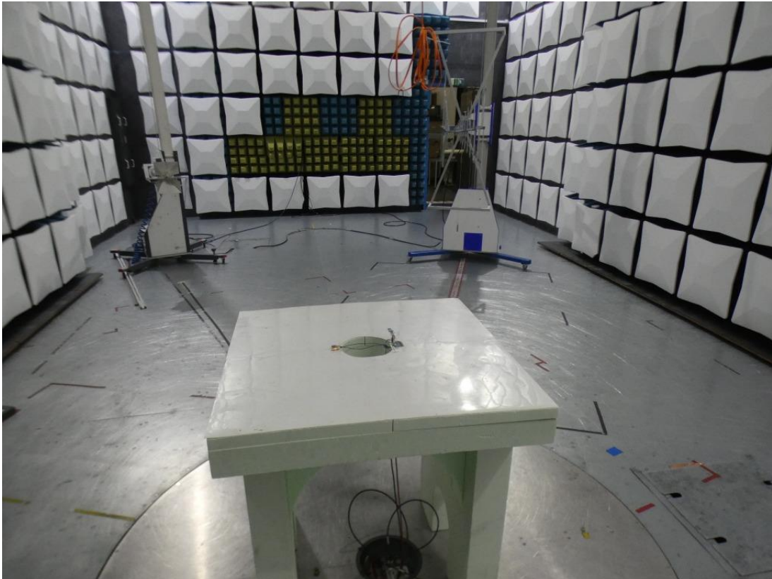
Photo 1: Test setup for radiated measurements below 1 GHz
