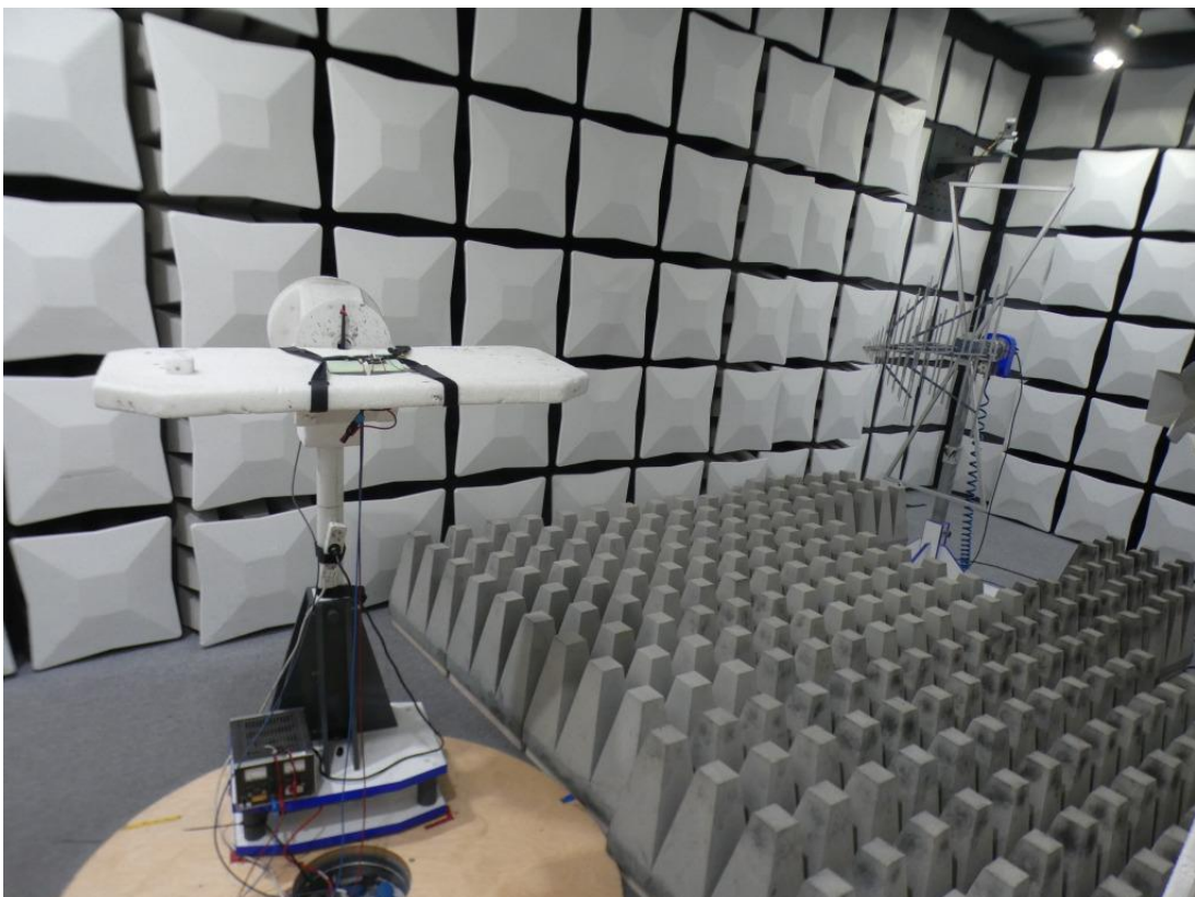
Photo 2: Test setup for radiated measurements above 1 GHz
