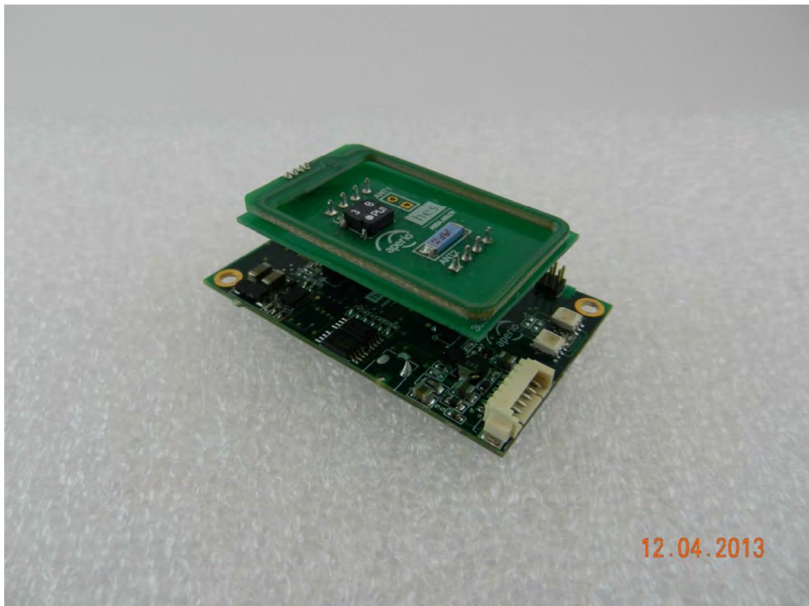
Antenna board mounted on main board
