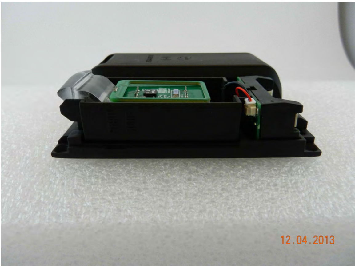
Side view (distance between antenna and cover = 1.5mm)
